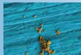
Traditional Urethane Pad Wiped Twice 6000 x Magnification
