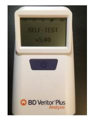
Analyzers with firmware v5.40 cannot be upgraded to v5.50
