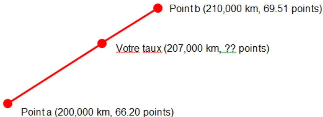
$$T_{ext} = T_a + (T_b - T_a) \times (km_b - km_{est}) \div (km_b - km_a)$$
