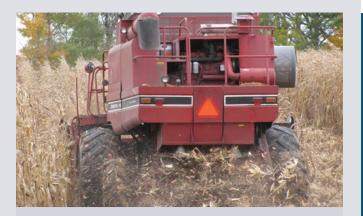
Spread residue evenly behind the combine to eliminate windrows and improve ground coverage to protect the soil.
