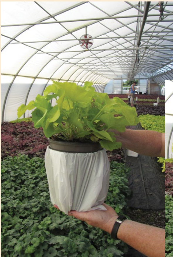
Use plastic-lined pots to measure % leaching fraction in each crop group. When combined with physical examination of media wetting front and root growth, %LF can be used to evaluate whether the volume of water applied at each irrigation event is too much or not enough.
