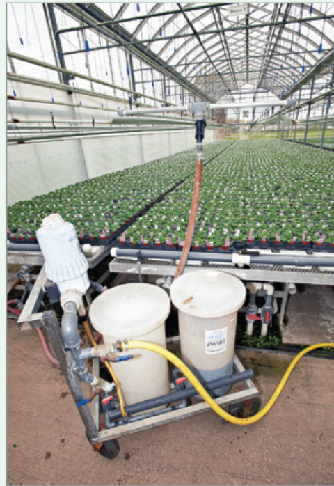
Flexible fertigation systems can match nutrients to crop specific needs, allowing for more efficient use of fertilizers.
