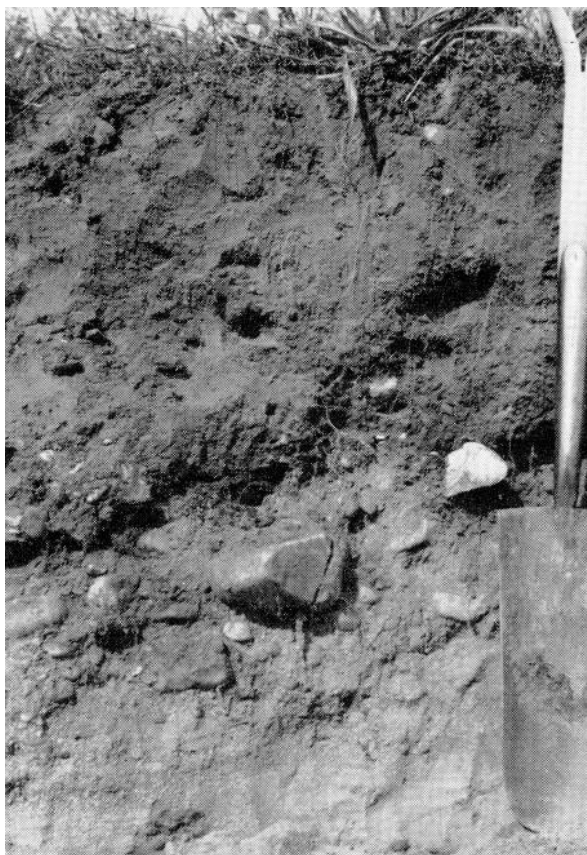
Profile of Grenville loam, a Brown Forest soil with a thin dark brown accumulation horizon occurring at the juncture of the solum and the calcareous parent material.
