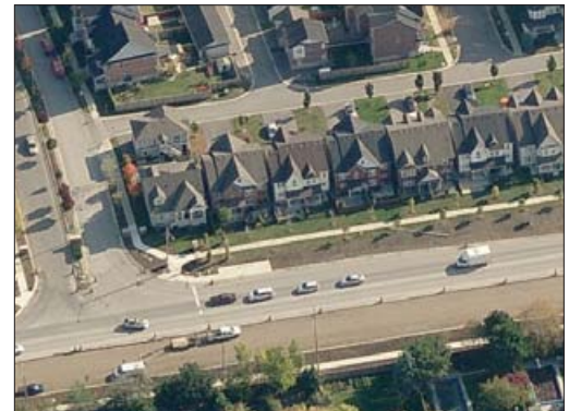
A rear access lane permits this housing in Markham to face onto a limited access arterial road.
