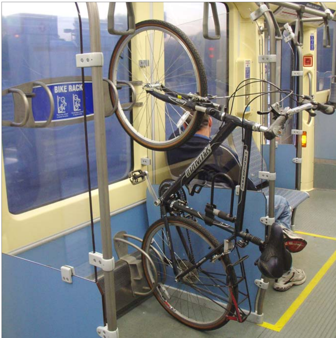
This LRT vehicle in Minneapolis has been designed to accommodate cyclists during all hours of the day.
