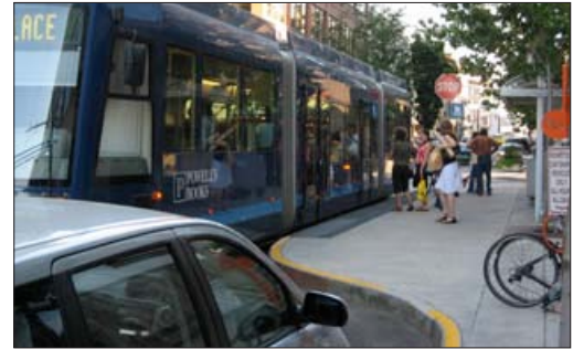
Bus-bulbs, such as this example in Portland, speed up boarding times while providing additional space in waiting areas.
