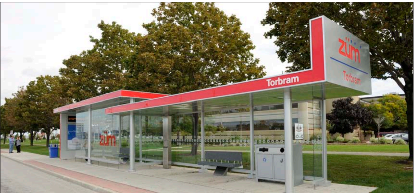
A heated bus shelter in Brampton provides real-time arrival information and provides waiting passengers with the choice of both internal and external waiting areas.
