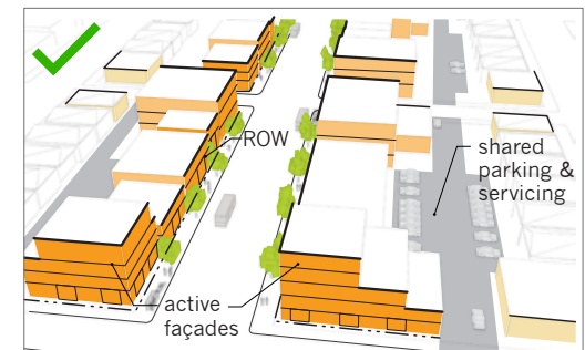
An undesirable building orientation (top) places entrances and active uses away from the street, while parking becomes the most visible element of the streetscape. A more desirable building orientation (bottom) places active uses and building entrances at the right-of-way (ROW), creating a continuous street wall and a more attractive pedestrian environment.
