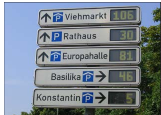
The use of real-time parking displays, such as this one in Germany, can help to maximise existing shared parking resources by informing drivers of the location of available spaces within a structure or district.
