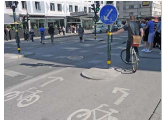
A dedicated bike crossing in Stockholm enables through cyclists to pass while turning cyclists are provided a place to wait for the appropriate signal.
