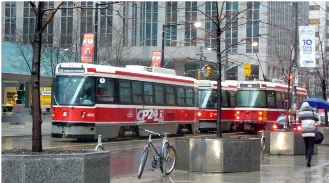
Bunching can delay vehicles and preclude any advantage that an increase in service might provide. Measures such as signal priority and automatic vehicle location can keep vehicles evenly spaced.
