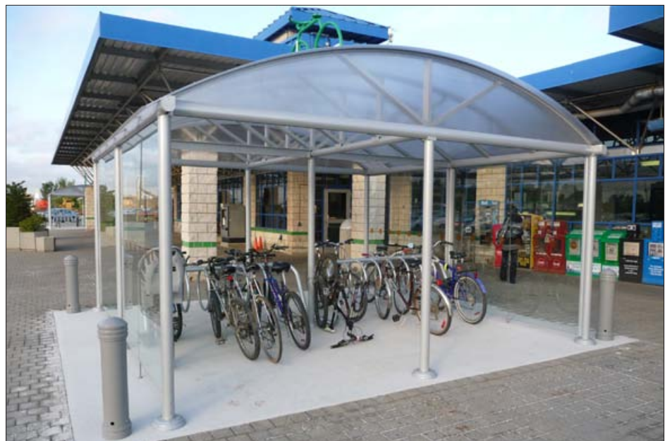
Sheltered bike facilities located in highly visible locations, such as this example in Oakville, help discourage vandalism and theft. The use of closed rings provides two points of contact for parked bicycles. This provides greater stability and makes it easier to lock the bike.
