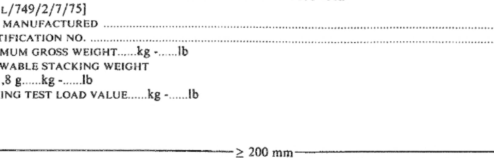
1 Country of Approval and Approval Reference as given in the example on line 1. (The country of Approval should be indicated by means of the distinguishing sign used to indicate country of registration of motor vehicles in international road traffic).
