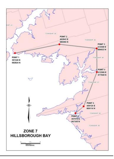
Points are referenced to the PEI Survey Reference System with all coordinates being expressed in metres. The projection (Double Stereographic), is referenced to the North American Datum of 1983 realized from the Canadian Spatial Reference System (NAD83(CSRS)).
